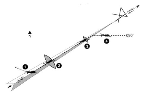
1. After establishing a localizer intercept heading with the heading bug while in HDG mode, the APR button is pressed. As APR coupling occurs, the APR annunciator light comes on steady, HDG light goes off, and the glideslope mode is automatically armed. The autopilot will roll the helicopter out on localizer and the course needle will center.
