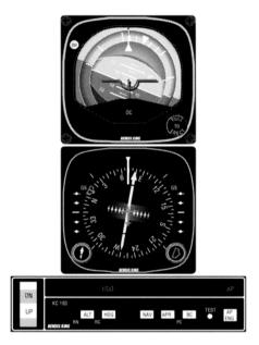
Desired altitude has been reached, altitude hold (ALT) has been engaged and the helicopter has returned to level flight. The 010 degree heading has been acquired.
