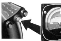
At the middle marker, the pilot disconnects the autopilot with the AP DISC button on the cyclic. This cancels all operating autopilot modes. The pilot initiates a missed approach.
