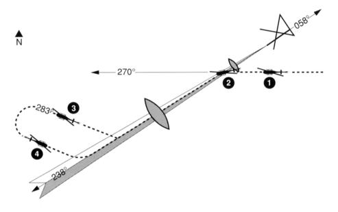
1. The helicopter is heading 270 degrees with heading (HDG), altitude hold (ALT) and autopilot (AP) engaged. To intercept and fly the ILS front course outbound, set the front course on the HSI and depress the Back Course (BC) button. The Back Course mode is selected to enable the autopilot to fly outbound on the front course. The capture point is now being computed based on closure rate.
