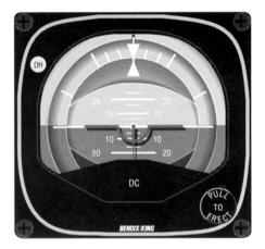
Erecting the KG 253 should only be accomplished while the helicopter is relatively level on the ground or in level flight. The gyro must be "up to speed" before system will operate. Allow three minutes for the gyro to come up to speed.
