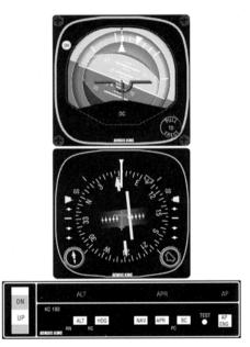
The autopilot follows the localizer, making automatic adjustments in heading to keep the course deviation needle centered. When the glideslope deviation needle reaches mid-scale, altitude hold is automatically disengaged when the glideslope is captured. The "ALT" light goes out and "GS" comes on. The autopilot will make pitch and bank changes as necessary to maintain glideslope and localizer tracking.
