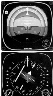
heading until entering the capture zone, then turn to intercept the course. The "HDG" light will go off and the "APR" light will illuminate steadily as the APR mode goes from arm to engage.
