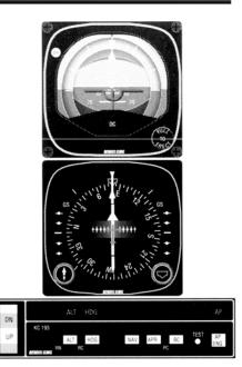
The helicopter has completed its turn to the 112 degree course. A wind correction produces a heading of 105 degrees, displaying a seven degree "crab" angle to maintain the 112 degree RNAV or Loran course.
