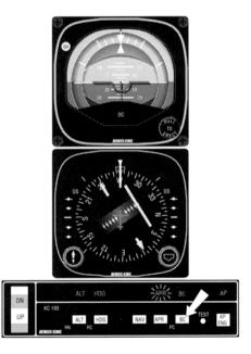
When the computed capture point is reached, HDG mode is cancelled, Back Course (BC) mode activates, and a left turn outbound on the localizer is initiated by the autopilot.
