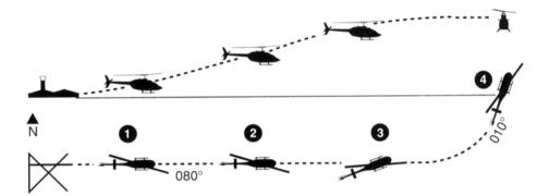
The helicopter is well off the ground and climbing with an appropriate airspeed.
