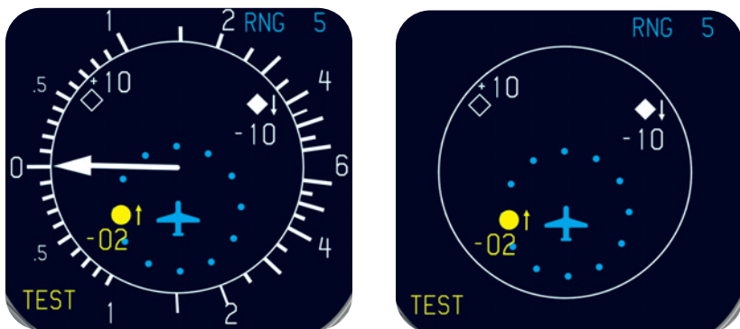
IVA 81A/C/D & TID 66A/D TCAS I Test Patterns; 5NM range
