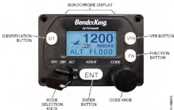
Figure 2-1 KGX Control Panel
